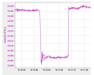
Figure 3. A typical salinity decrease when the plastic rod is placed near the conductivity cell. The data shown above is acquired with a plastic rod (d=2.54cm) placed 1cm away from the conductivity cell.
