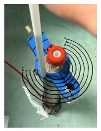
Figure 2. Experiment setup. The rod in this photo has an OD of 1.27cm and is placed 1cm away from the conductivity cell.
