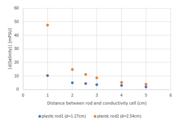
Figure 4. A scattered plot to visualize the results presented in Table 1. The x-axis is the distance between the plastic rod and conductivity cell in cm, the y-axis is the absolute value of salinity difference in mPSU.
