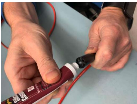
Fig. 15. Applying silicone compound to the female connectors.
