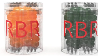
Fig. 11. Fresh (orange) and saturated (green) desiccant capsules.
