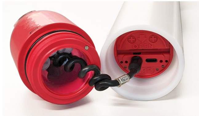
Fig. 4. Open instrument with a connectorised end-cap
