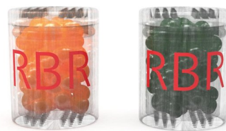
Fig. 19. Fresh (orange) and saturated (green) desiccant capsules.
