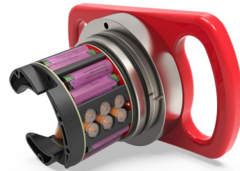
Fig. 14. Location of the batteries
