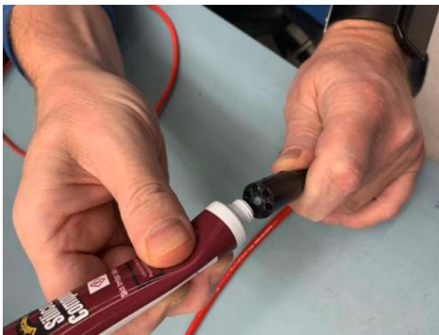
Fig. 17. Applying silicone compound to the female connectors.
