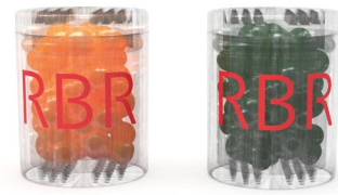
Fig. 16. Fresh (orange) and saturated (green) desiccant capsules.
