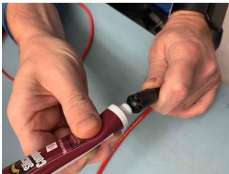
Fig. 16. Applying silicone compound to the female connectors.
