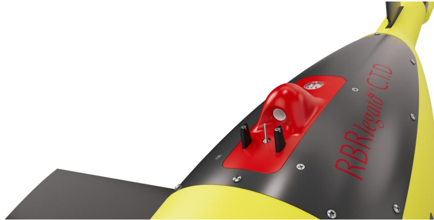
Fig. 1. An RBRlegato 4 installed in a glider.
