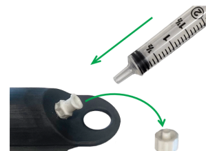
Fig. 14. Gently push down the piston to inject until full.
