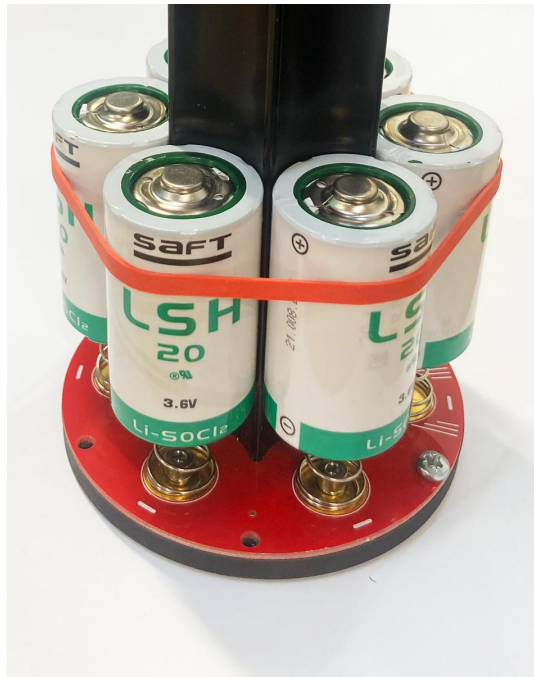
Fig. 7. Lithium batteries retained in assembly
