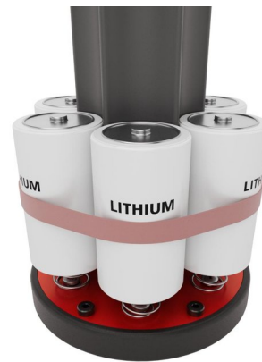
Fig. 5. A view of lithium batteries held in to the carousel using a red retention band.
