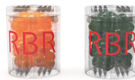
Fig. 11. Fresh (orange) and saturated (green) desiccant capsules.
