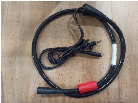
MLM test loop cable
