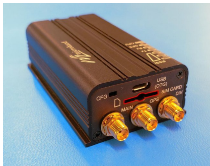
Fig. 31. GSM/RUDICS dual modem pre-April 2021
