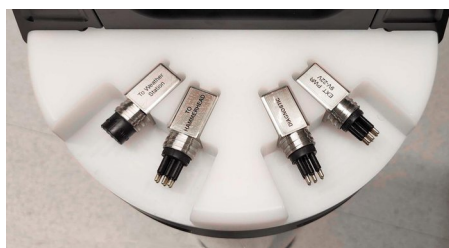
Fig. 4. RBRcervello with four wired connectors
