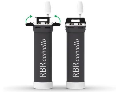
Fig. 8. Closing the locking tabs (RBRcervello, dual modem)
