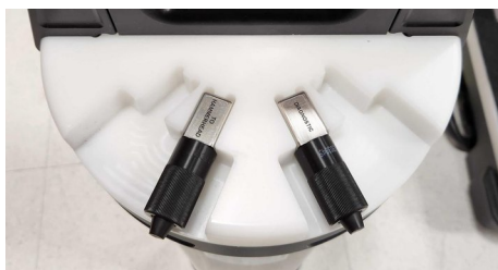
Fig. 3. RBRcervello with two wired connectors
