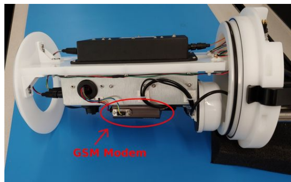
Fig. 33. RBR cervello , GSM/RUDICS dual modem, pre-April 2021
