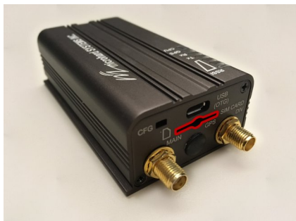
Fig. 30. Legacy GSM modem, isolated with the SIM-card slot highlighted
