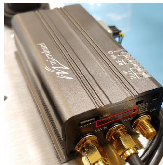
Fig. 32. GSM/RUDICS dual modem post-April 2021
