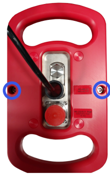
Opening screws, torqued to 1.7Nm
