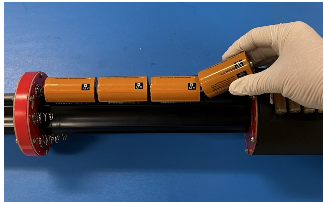
Batteries' positive terminals face the battery end-cap
