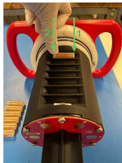
Insert desiccant canisters end-first
