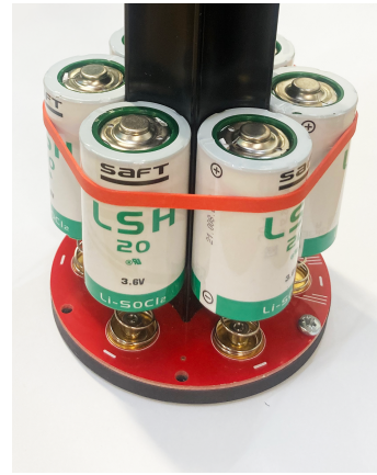
Lithium batteries retained in carousel
