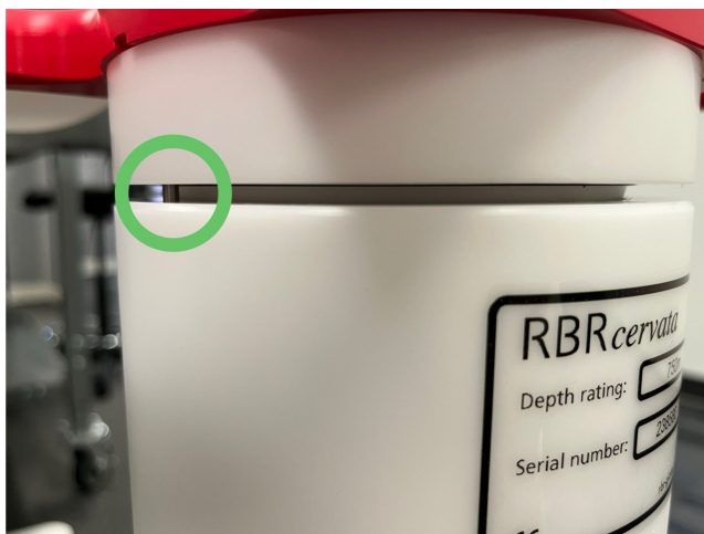
The alignment pin partially seated in its hole
