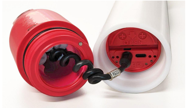
Fig. 10. Open instrument with a connectorised end-cap
