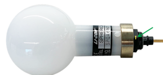
Fig. 25. The LI-COR PAR sensor: note the location of the yellow mark
