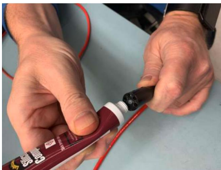
Fig. 30. Applying silicone compound to the female connectors.
