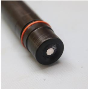
1. Twist off the black cap. We recommend that you unscrew the cap with the sensor facing downwards to ensure the electrolyte fluid remains inside the cap. (See *image A*)
