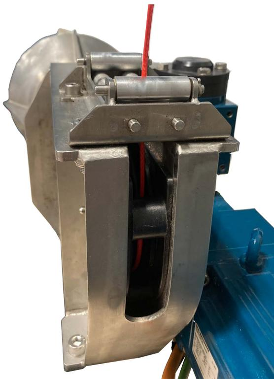
13. Pull the line in front of the line tensioner rollers and out of the bell mouth. Hold the end of the line with your hand for the following step.
