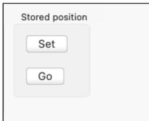
1. When the instrument is in the bell mouth, click **Set**. This will be the zero position for your instrument.
