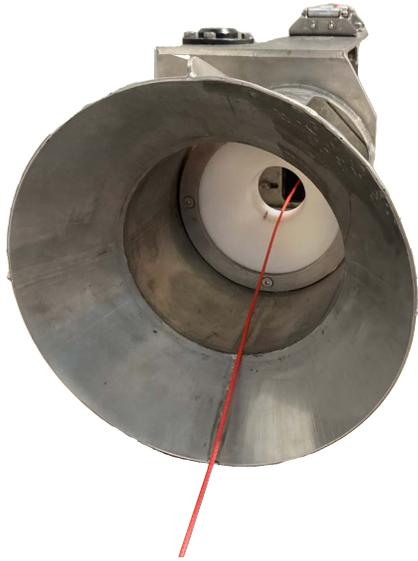
**⚠** The two tensioner rollers are sitting very snug, so leave the line outside the point where they touch. Once the winch starts moving, the line will be drawn in between the rollers.
