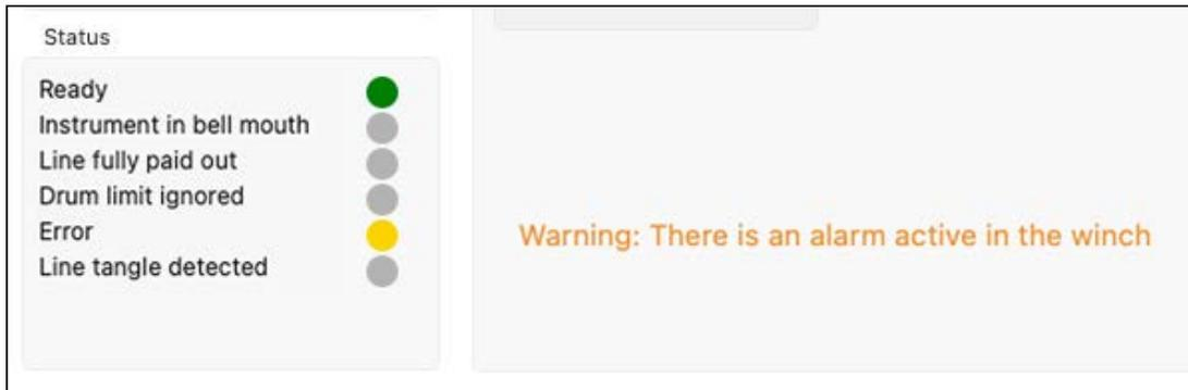
**Solution:** Turn the winch off and on again to clear the error.
