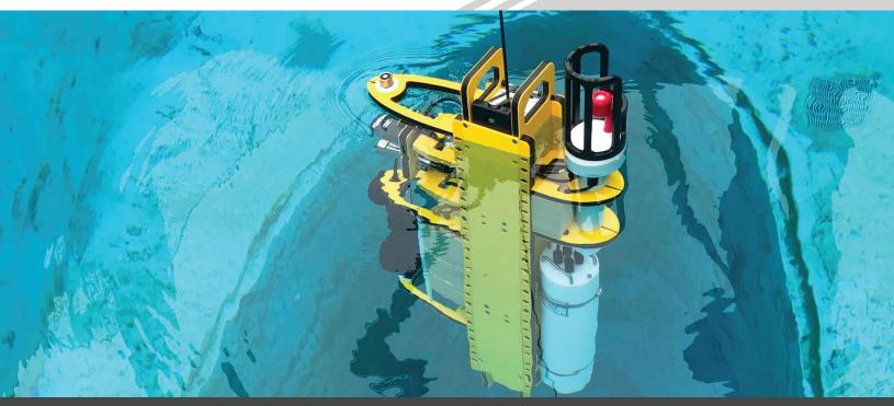
RBR is pleased to offer the Del Mar Oceanographic WIREWALKER™, a wave-powered profiling system where mechanical, sensing, and communication elements are all tightly integrated. The DMO WIREWALKER™ can be configured using either the RBRconcerto<sup>3</sup> or RBRmaestro<sup>3</sup> instruments.
