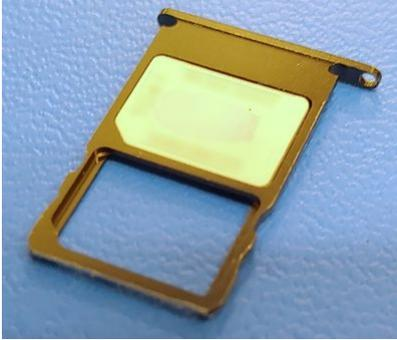
5. Insert the tray with the SIM-card installed and its electrical contacts facing downward. Handle it with care to prevent the SIM from falling out of the tray.
