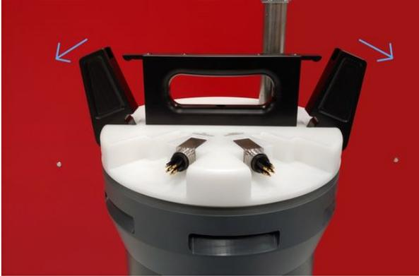
3. Rest the internal assembly on the lip of the housing.
