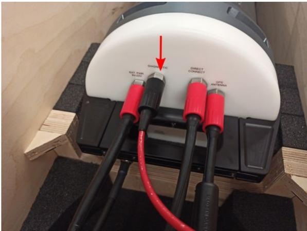
2. Follow the steps in [Using the diagnostic port](#) to set up the terminal and access the RBRcervello's menu.
