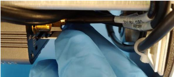
6. Push the tray in until flushed with the modem's chassis. Avoid moving the RBR*cervello* until the tray is fully inserted to prevent the SIM from falling out of place.
