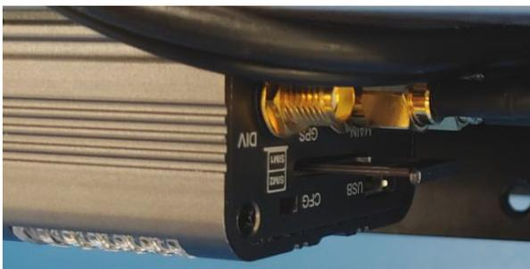
4. Put the micro SIM-card into the SIM1 position, with the electrical contacts facing down.
