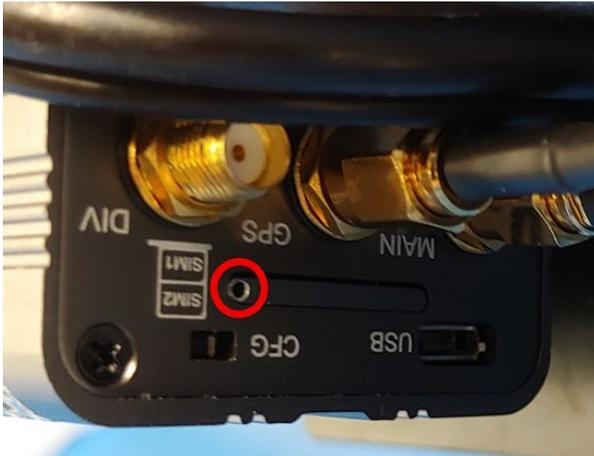
2. Insert the SIM removal tool as straight as possible into the pinhole and push. The tray will pop out.
