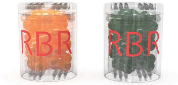
Fresh (orange) and saturated (green) desiccant capsules
