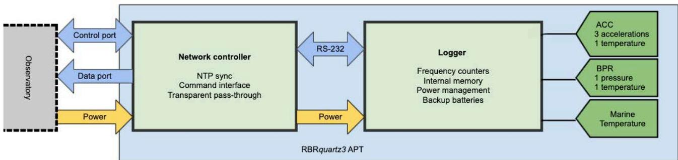
**i** You do not need to open your instrument to connect it to your network. Connect your terminal to the MINK port located outside the instrument body using a compatible MINK cable. The instrument will appear on your network.
