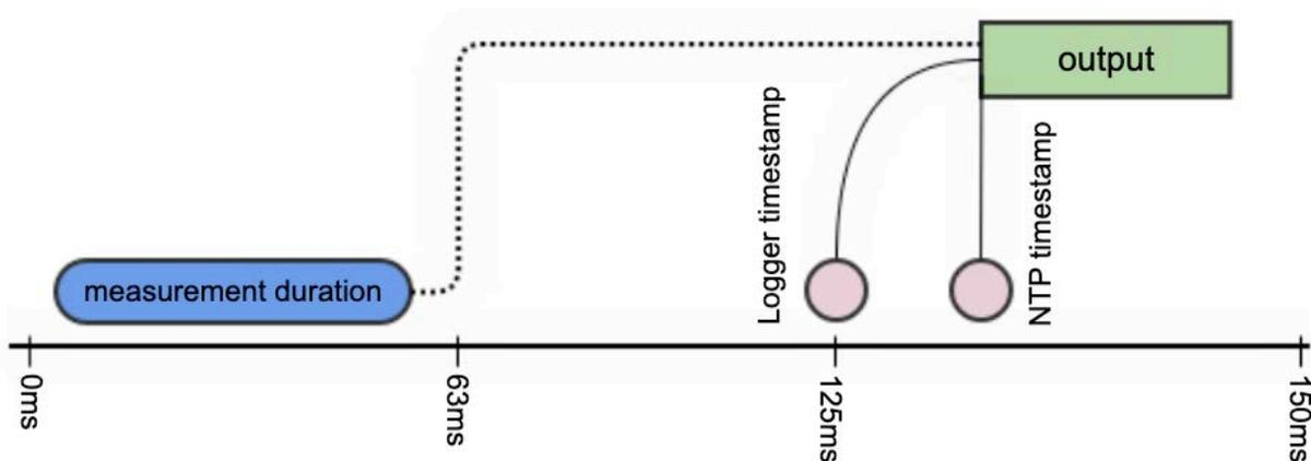
Logger readings will be timestamped no earlier than 63ms and no later than 125ms from when the reading was completed. The resolution of logger timestamps is 63ms. Logger output of the timestamped sample will occur within 63ms of the indicated timestamp.
