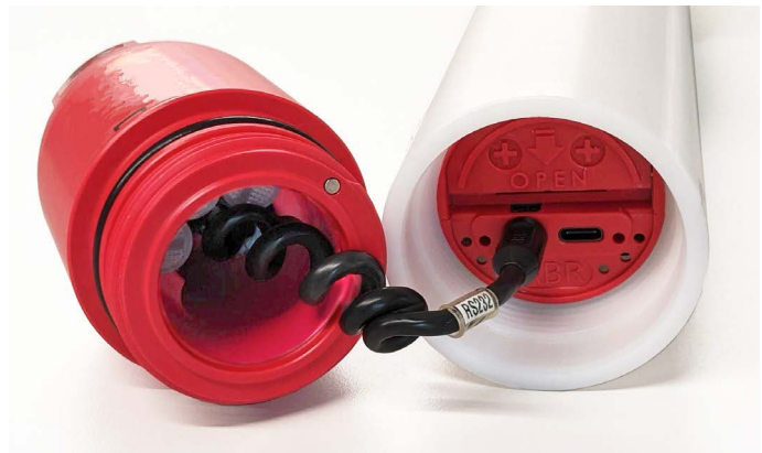
Open instrument with a connectorised end-cap
