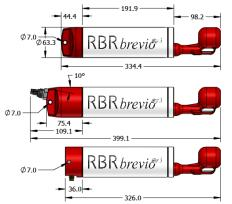
RBR*brevio*<sup>3</sup> dimensions with three different battery end-caps
