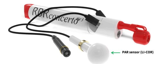
RBRconcerto<sup>3</sup> C.T.D.DO.PAR with a spherical PAR sensor (LI-COR)
