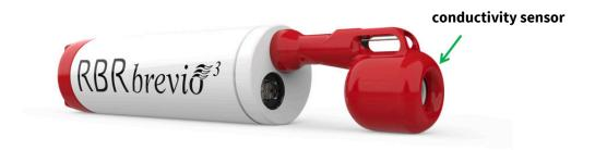
RBR*brevio*<sup>3</sup> C.T.D with a conductivity sensor
