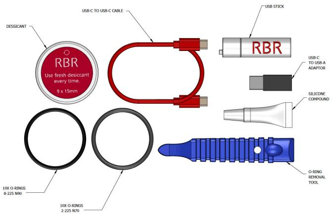
**RBR support kit diagram (for titanium)**
