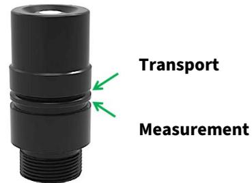
During transportation or storage, move the red O-ring of the Oxyguard sensor to the "Transport" position, closing off the port on the side of the cell.
