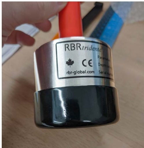
RBRtridente with its storage cap on
