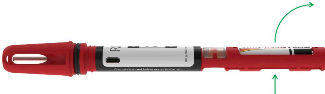
Push the old battery out
