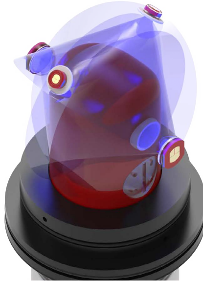
Four UV LEDs illuminating the CT cell
