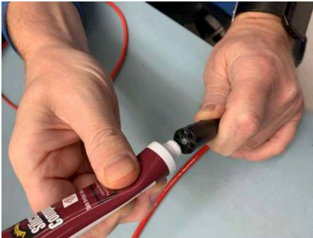
Lubricating a connector
