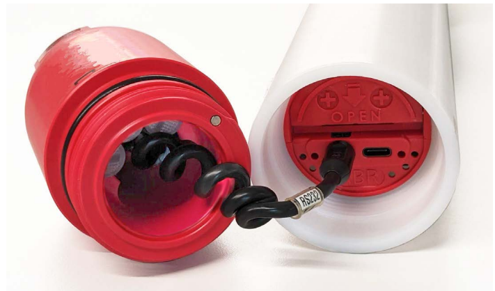
Open instrument with a connectorised end-cap
