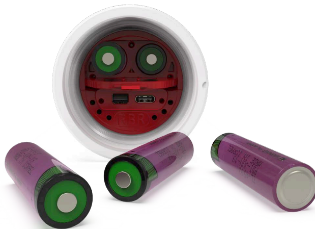
RBR standard instrument with batteries removed
