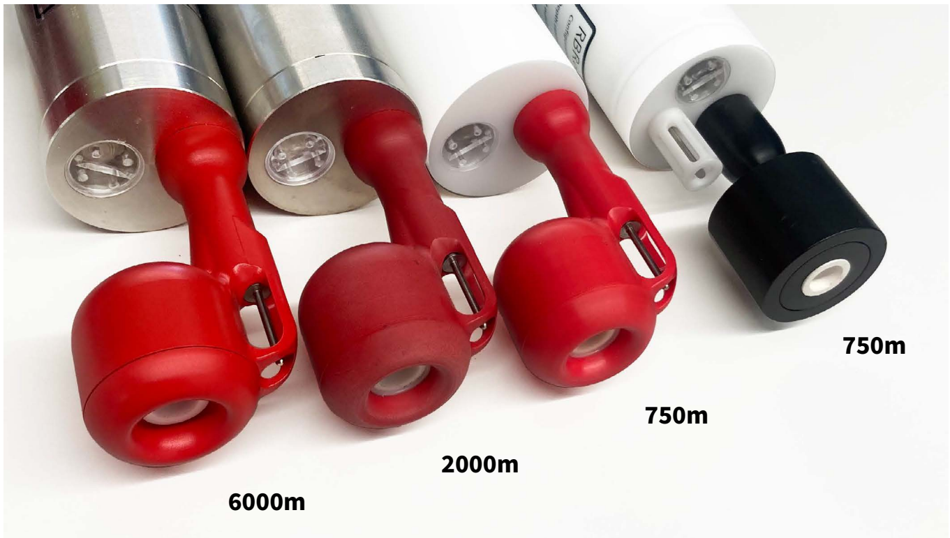
750m-, 2000m-, and 6000m-rated conductivity cells
