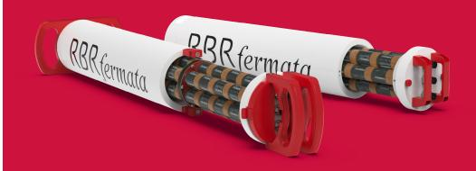
The RBRfermata battery canister extends deployments of all instruments by providing up to 2.8kWh of energy to any underwater instrument, which is about forty times greater than our standard battery carriage capacity. Housing 48 individual D-cells and hosting three MCBH connectors, it has both a 14V and 28V option. An innovative battery carrousel coupled with quick-release or low-profile handles facilitates simple, tool-free battery replacement.
