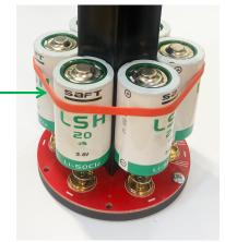
Note: Always remove the batteries from the canister during long-term storage! Doing so will prevent internal damage due to battery leakage and/or corrosion.
