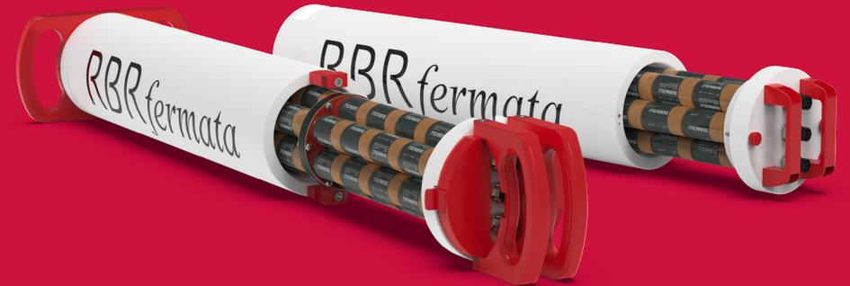
The RBRfermata battery canister extends deployments of all instruments by providing up to 2.8kWh of energy to any underwater instrument, which is about forty times greater than our standard battery carriage capacity. Housing 48 individual D-cells and hosting three MCBH connectors, it has both a 14V and 28V option. An innovative battery carousel coupled with quick-release or low-profile handles facilitates simple, tool-free battery replacement.
