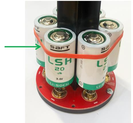
*Note: Always remove the batteries from the canister during long-term storage! Doing so will prevent internal damage due to battery leakage and/or corrosion.*
