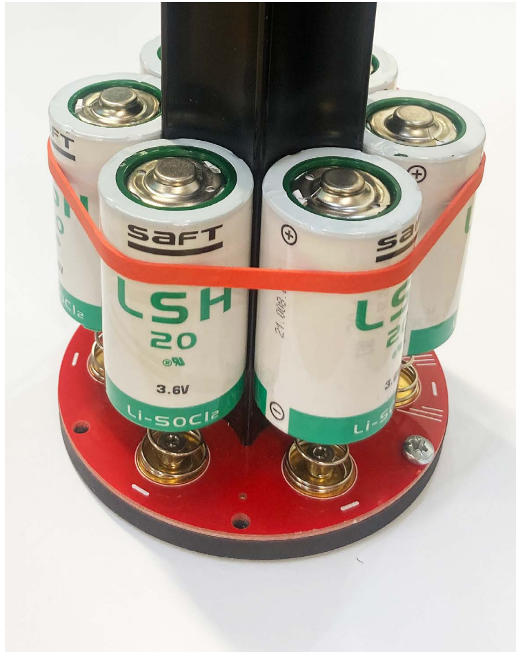
Lithium batteries retained in assembly
