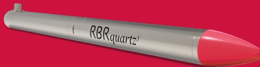
The RBRquartz<sup>3</sup> APT (Accelerometer, Pressure, Temperature) combines a triaxial quartz accelerometer with the Paroscientific Digiquartz<sup>®</sup> pressure sensor, building on the capabilities of the RBR bottom pressure recorders. The RBRquartz<sup>3</sup> APT supports both autonomous installations and realtime data streaming to cabled observatories. The external ports may be configured as either USB, RS-232/RS-485, or Ethernet (selected at the time of order).
