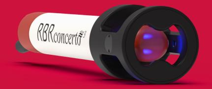
The RBRduo³ C.T|uv and RBRconcerto³ C.T.D|uv offer the same features as our trusted conductivity, temperature, and depth instruments, plus active antifouling. Four UV LEDs illuminate critical sensor surfaces and control biological growth on the conductivity cell, thus maintaining high accuracy measurements during extended deployments in the photic zone.
