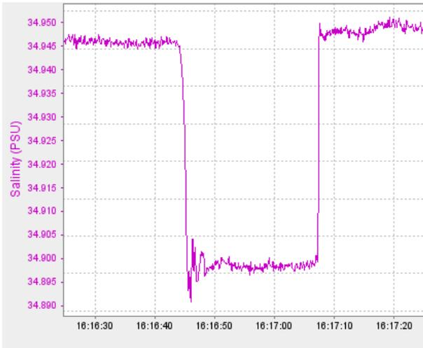
Figure 3. A typical salinity decrease when the plastic rod is placed near the conductivity cell. The data shown above is acquired with a plastic rod (d=2.54cm) placed 1cm away from the conductivity cell.
