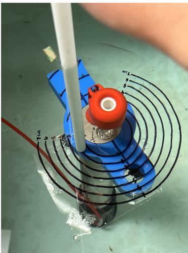
Figure 2. Experiment setup. The rod in this photo has an OD of 1.27cm and is placed 1cm away from the conductivity cell.
