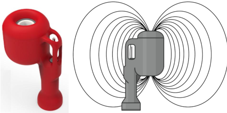
Figure 1. On the left, a 2000dbar CT cell. On the right, an illustration of the current field lines of the conductivity cell.
