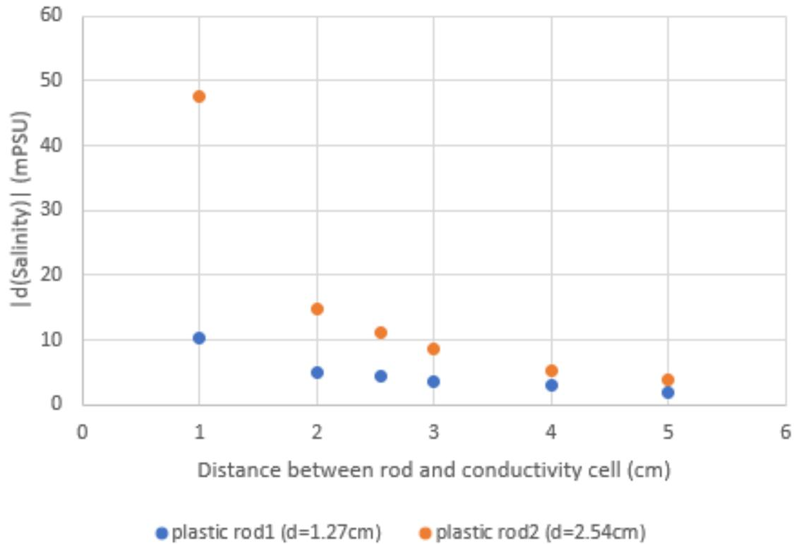
Figure 4. A scattered plot to visualize the results presented in Table 1. The x-axis is the distance between the plastic rod and conductivity cell in cm, the y-axis is the absolute value of salinity difference in mPSU.
